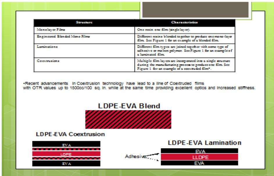
Since gases will move through each independent layer sequentially, the OTR of each independent layer of polymer must be determined and inserted into the following equation to calculate the overall structure oxygen transmission rate (see **Figure 4**).
