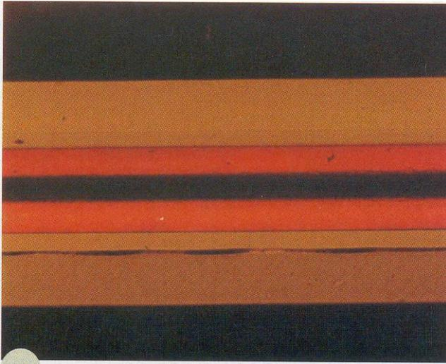
**Fig. 1**—Cross-section of a 7-layer barrier material photographed using 200× magnification
